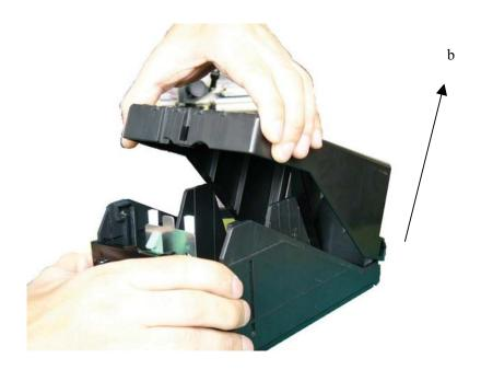
(3) Pull the pressure plate toward you and raise it along the grooves on both sides. When the pressure plate reaches the top of the groove, push the pressure plate forward so that it can be settled in the slots leading out of the grooves.
