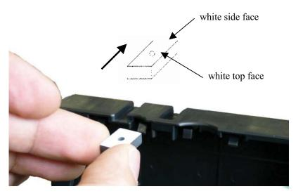
\*Make sure that denomination magnets are completely fitted into slots under a claw.
