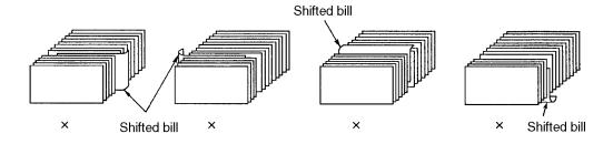
(3) Load bills in staggered units of 100 sheets so that the stack of bills does not bulge.
