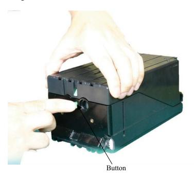
(2) Lift the lid up in the direction of arrow "b" to completely open the cassette.
