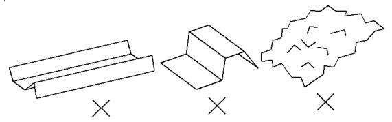
(8) Do not use the bills having serious wrinkles or broken section wherein paper fiber is broken and separation begin. Broken section
