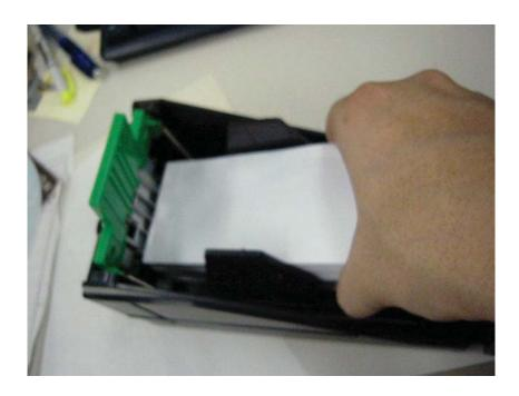
(6) Lower down the pressure plate to hold the loaded bills.
